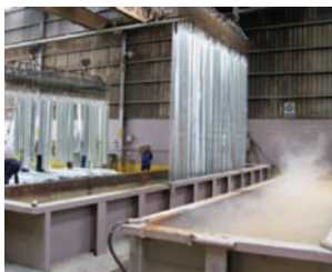
Counter-current rinsing can typically be used in electroplating operations
